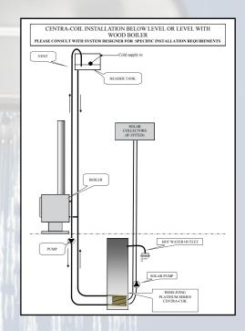
Combined with hydronic radiator or infloor heating systems, the centra-coil can be on a continuous heating cycle with the home heating or on a priority heating via a simple wise logic control system.
