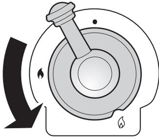
OFF position and wait one minute, then try again this time holding in the control knob for slightly longer.
