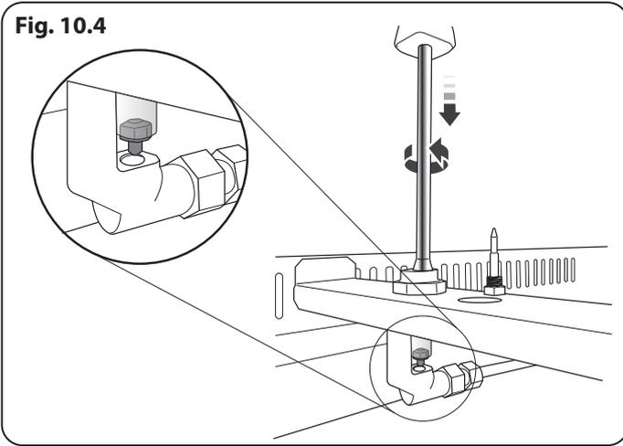
Save the orifices removed from the appliance for future use.
