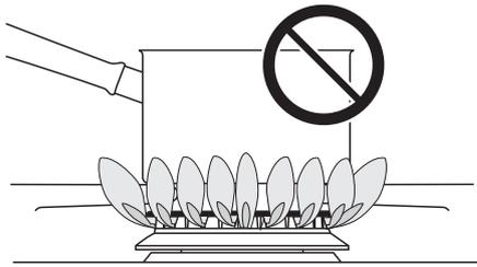
Pans and kettles with concave bases or down-turned base rims should not be used (**Fig. 2.5**).
