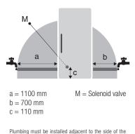
appliance which contains the locMaker. Water pressure must be between 0.15 MPa and 0.6 MPa (1.5 bar - 6 bar)
